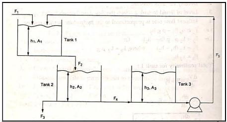
All the flow rate are volumetric and cross sectional area of three tanks are  $A_1$ ,  $A_2$ ,  $A_3$  (m<sup>2</sup>) respectively. The flow rate  $F_5$  is constant and does not depend upon  $h_3$ , while all other effluent flow rates are proportional to the corresponding hydrostatic liquid pressure that causes the flow.
